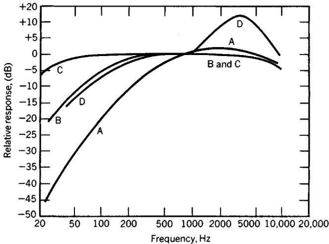
Fig. 29.7 Frequency characteristics for weighting functions of sound level meters.
