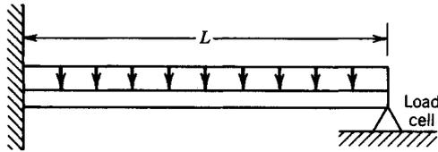
Fig. 29.3 Measuring the reactive force at the tip.
