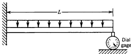
Fig. 29.4 Measuring the tip deflection.
