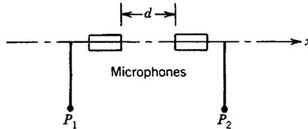
Fig. 29.9 Intensity measuring probe.
